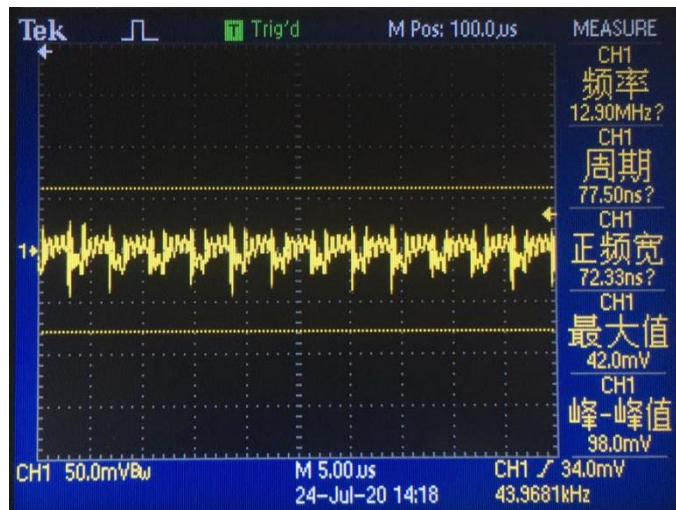
Noise ( V_{IN} = 48V , I_O = 0.6A , 5 ~ 20MHz bandwidth)
