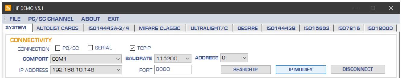
After the connection is established, click on [IP MODIFY]. This will open a dialog box to configure the Ethernet interface.
