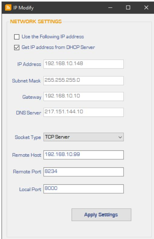
The standard setting of the socket type is TCP Server. This means that a control software connects with the RFID device. The connection is made with the Local Port.
